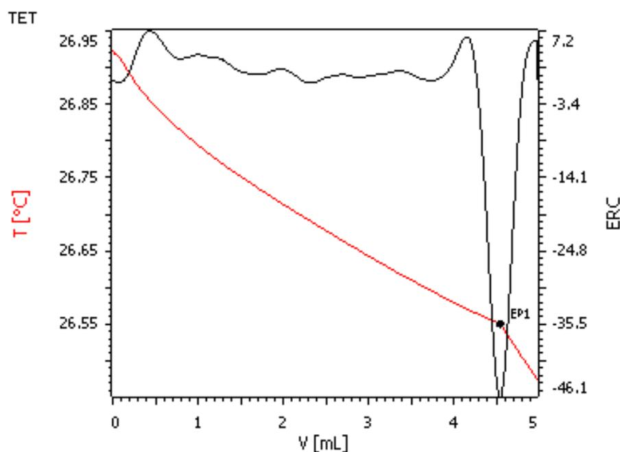
Hydrogen peroxide solutions may be determined by an iodometric thermometric endpoint titration (TET). Iodide is oxidized to iodine, which is reduced exothermically by standard sodium thiosulfate titrant.
