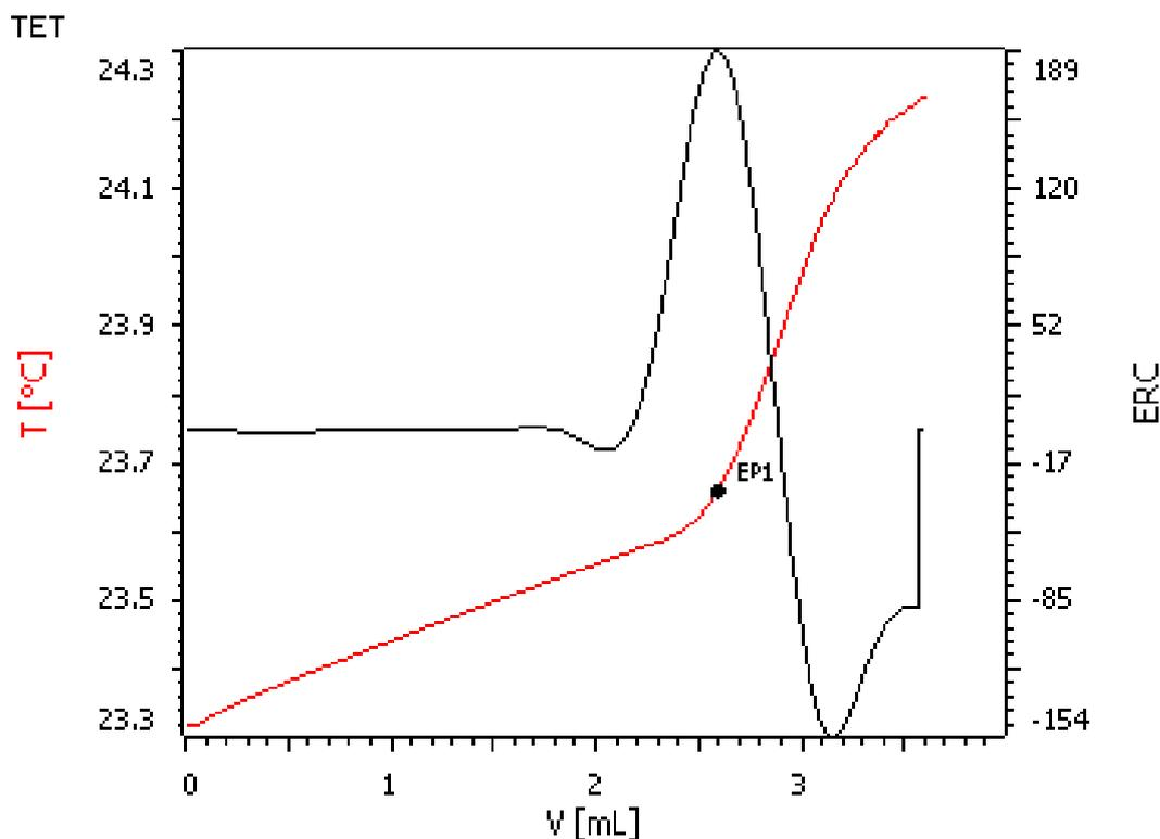
This Application Note covers the determination of aluminum in silica-containing samples with EDTA using thermometric titration. Excess EDTA is titrated with a known concentration of  $\text{Cu}^{2+}$  ions. First traces of  $\text{Cu}^{2+}$  cause the  $\text{H}_2\text{O}_2$  in the solution to decompose very rapidly, which is indicated by a sudden temperature increase.
