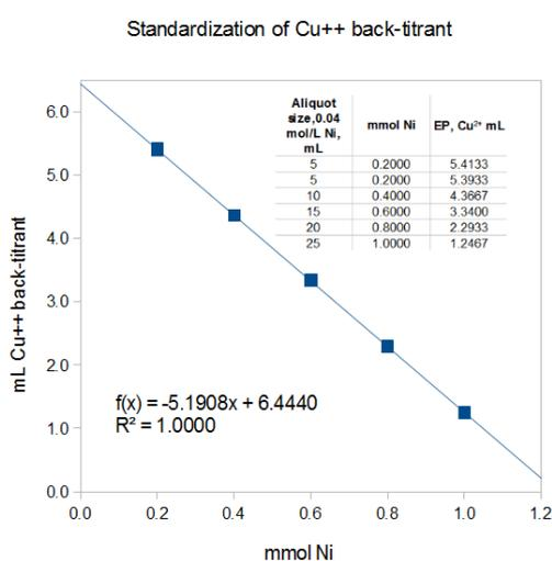
Regression analysis of standardization of Cu<sup>2+</sup> back-titrant solution with standard 0.04 mol/L Ni<sup>2+</sup> solution
