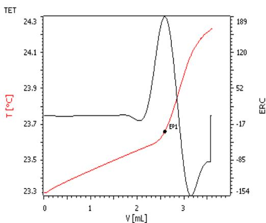
Back-titration of Al<sub>2</sub>(SO<sub>4</sub>)<sub>3</sub>·16H<sub>2</sub>O
