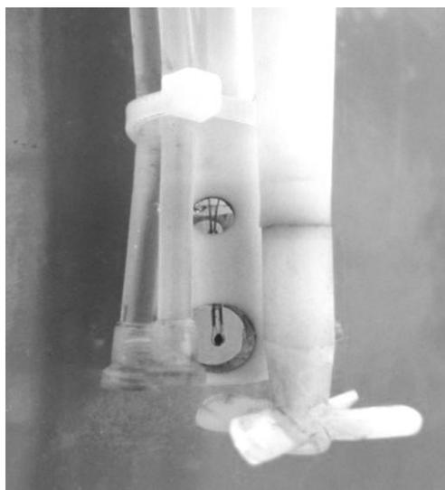
Optimal arrangement of titration head for use in 75 mL titration tubes. Note titrant delivery tubes are lower than the Thermoprobe.
