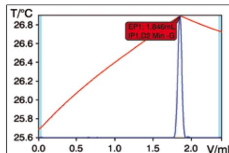
**Fig. 3:** Example of the determination of the fluoride content of a solution consisting of a mixture of hydrofluoric acid, ammonium hydrogen difluoride and acetic acid by thermometric titration.
