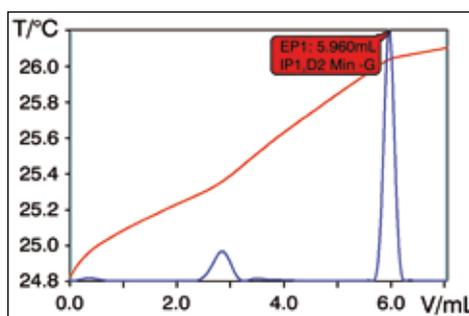
**Fig. 2:** Titration curve and its second derivative for the determination of the aluminum content of an aluminum chloride solution by thermometric titration.
