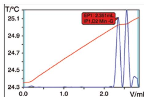
Fig. 1: Determination of the sodium content of a grill sauce.
